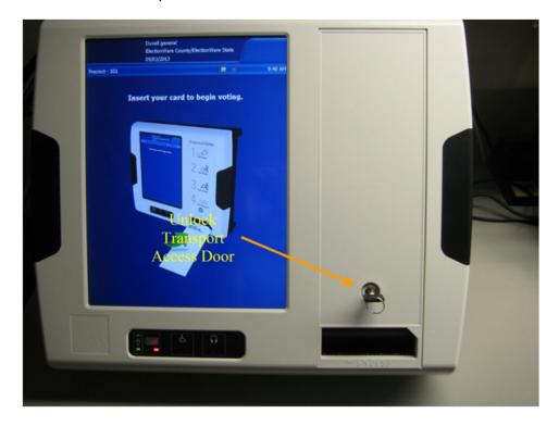
2. Open the transport access door. The prop rod supports the door in the open position.
