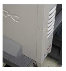
2. Press down on the front panel and then slide it off as shown in the picture on the right.
