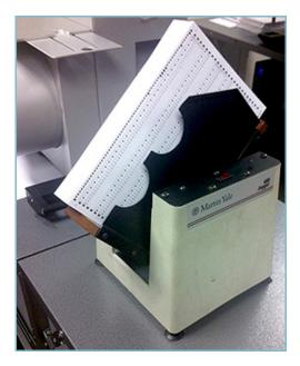
While back-bending the ballots, ensure that the folds line up (see "Correct" image below), and that the outer ballot does not wrap around the stack (see "Incorrect"). Bending the stack harshly with the ballots wrapping can introduce an additional fold and the unwanted "stair-step."
