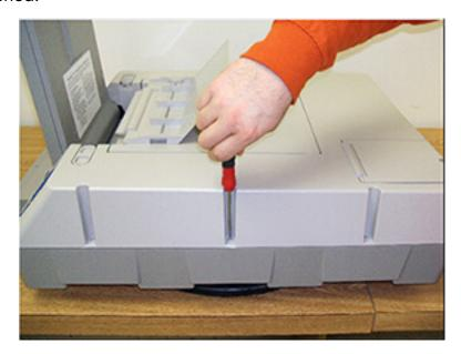
2. Remove the four screws on the inner edge of the top cover. There are two on each side.
