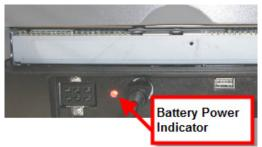
• If the light is flashing green, the battery is charged.
