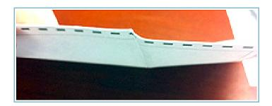
Alternately, ballots folded together in a Z or Map fold pattern have significantly fewer issues with rounded bends.
