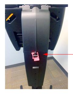
A seal here secures the container door. Leave in place during voting.
