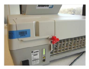
Additional seals can be used on the AutoMARK to prevent unauthorized access to the SBC casing and USB port. Only an ES&S-certified technician or trained vendor technician should apply these seals.
