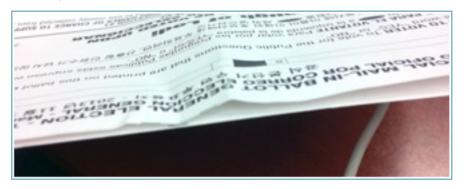
When such ballots are scanned with a DS850, they should be run with the undamaged edge leading and the damaged edge trailing.
