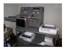
The Model 650 (M650) Central Ballot Counter with the two printers connected. The M650 uses the similar optical mark sensor design as the M550 but has a straight through ballot feed path to a receiver bin to the side. The M650 is a faster counter than the M150 or M550. See the detailed Specification sheet for more details. The M650 is based on QNX 4.25 operating system.
