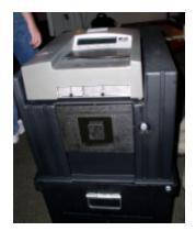
The Model 100 (M100) Precinct Ballot Counter mounted on Ballot Box. See detailed Specification sheet for more details. The M100 is based on the QNX 4.22 operating system and uses an Intel 286EX Processor. The optical sensor is sensitive in the visual light spectrum and detects changes in marking across the page as the ballot passes under the scan head. The device is programmed to recognize ballots common to the M150/550/650 line of ballot scanners and can take the ballots in any orientation.
