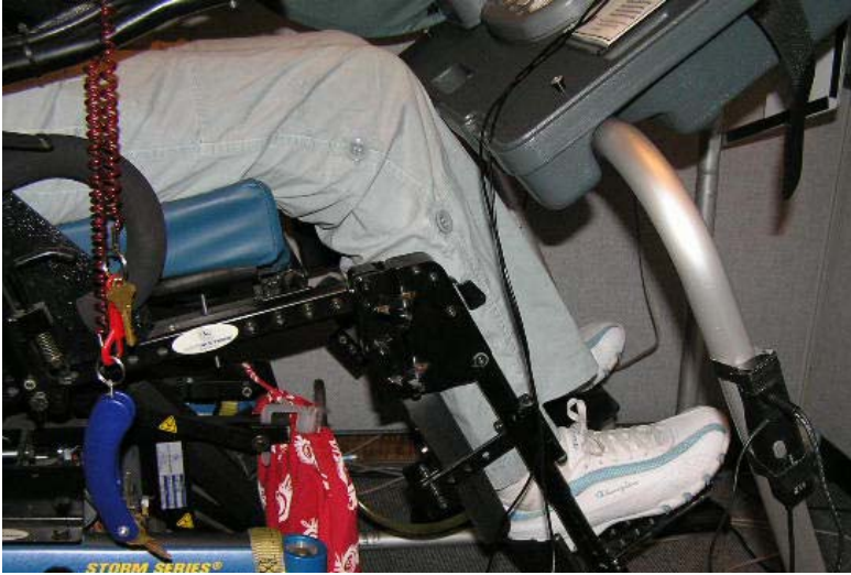
The user's knees meet the bottom of the eSlate while the user is still out of range of the controls.
