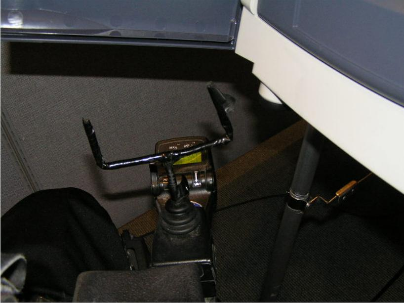
The lower edge of the machine is too close to the wheelchair control when this user approaches from the right.
