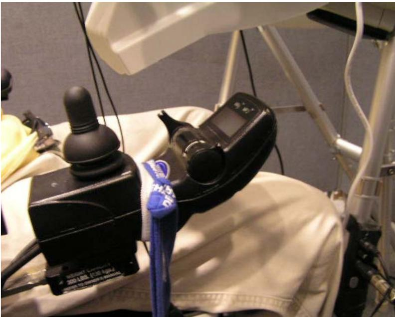
Side view of the same wheelchair control approaching the Diebold; the VVPAT interferes with the joystick.
