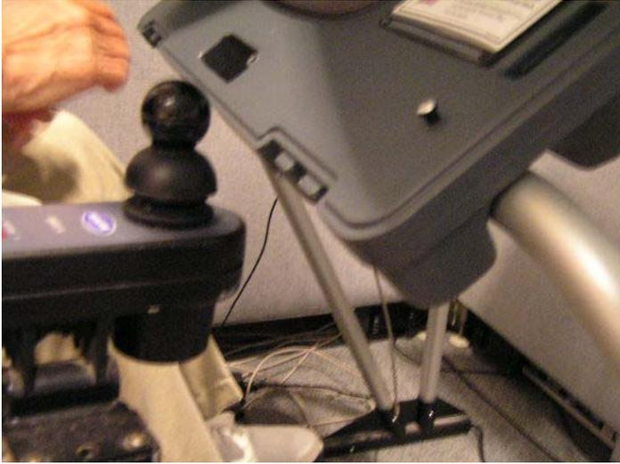
The bottom edge of the eSlate interferes with the wheelchair joystick and even with the armrest.
