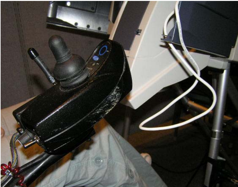
This wheelchair control juts forward of the right armrest. The Diebold VVPAT prevents enough forward progress for the user to reach the touch screen.
