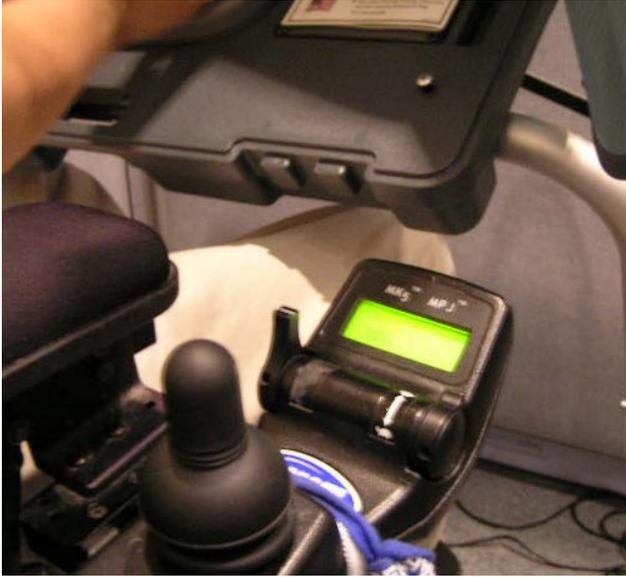
The front part of this wheelchair control barely makes it under the bottom edge of the eSlate; that edge is too low for the joystick itself.
