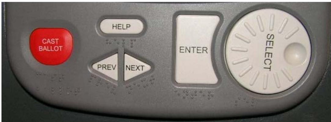
The controls of the Hart eSlate are built into the tablet, all along the lower edge directly beneath the screen. At the extreme right is a rotating Select wheel (radius = 31 mm). The wheel has radial ridges and a single dished depression for a finger or mouthstick. To its left is the Enter button, 50 mm tall by 32 mm wide,
